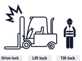
The OPSS System restricts driving, lifting and tilting, and it kicks in automatically when the operator leaves the seat to prevent accidents. It operates in conjunction with the auto parking brake to contribute to a safer workplace.
