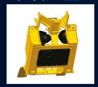
This recycling option includes a **floor cover and rear wheel-archer cover** in order to keep the engine bay free from debris or dirt. **This option protects all vital components such as the engine's radiator.**
