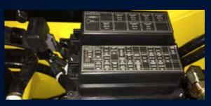
All fuses and relays are centralised in three boxes with **enhanced waterproof and dustproof protection IP65**. The boxes themselves are located under the foot panel for **quick access**.
